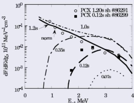
Numerical simulations of NPA in TFTR: more effects are included: (1) realistic geometry, (2)  $S = S(v, t)$  (Gorelenkov, NF'97)
